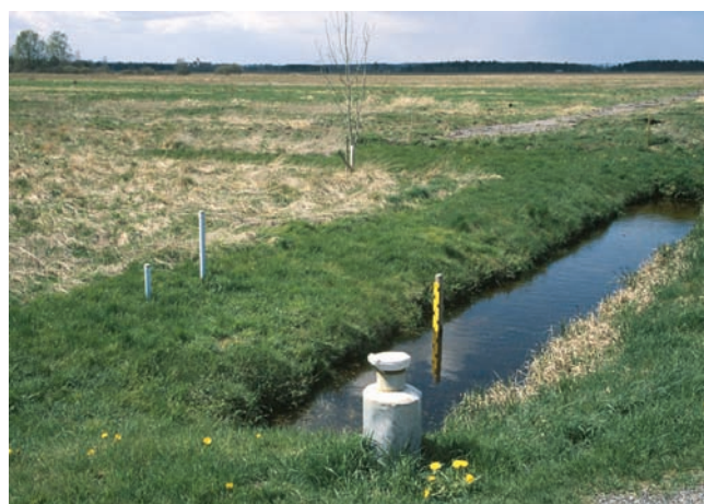
Groundwater level measuring stations monitor the groundwater tables in an area of the Federsee bog, which has undergone wetland restoration. The archaeological evidence remains preserved beneath the peat cover. Photograph: Stuttgart Regional Council, H. Schlichtherle.
