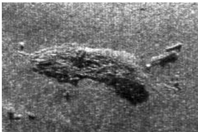
Figure 2: Side scan sonar image of the wreck of the Faro A
