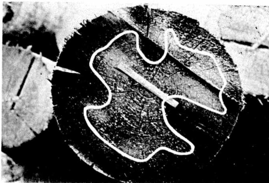
Fig. 8. Preservative penetration in roundwood and timbers is seldom complete. Instead a treated shell surrounds the untreated core.
