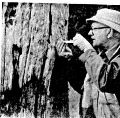
Fig. 27. Hugh V. Martin, MacMillan Bloedel Research Laboratory, Vancouver, B.C. taking depth of penetration measurements on the tangential surface of the totem pole with a spring steele vernier depth gauge. Credit Ruth Kirk, Tacoma, Washington.
