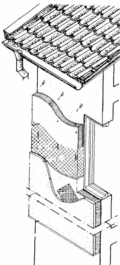
**Fig. 11.** Thermal insulation with plaster according to the Swedish Serporock method. Mineral Rock is attached to the wall with clasps and then plastered. The plastered mineral wool and the wall can then expand and contract independently.
