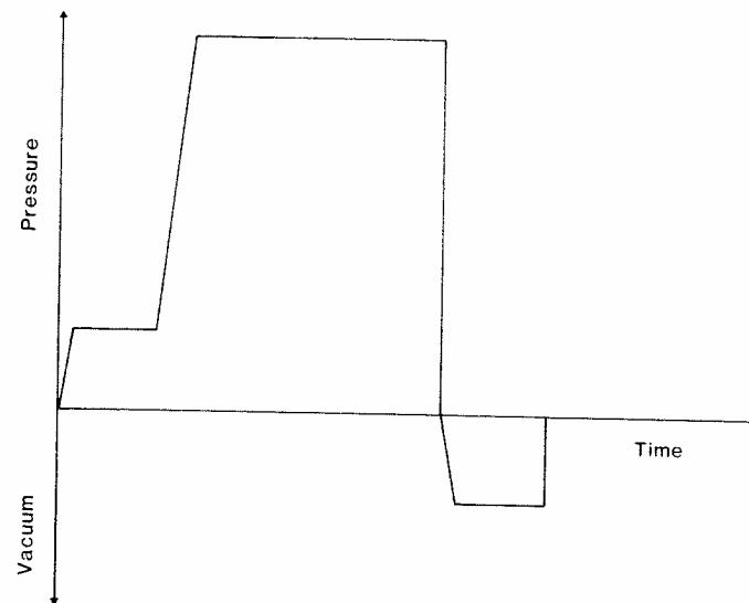
Fig. 14. The two empty cell processes used in North America are a) the Lowry Process and b) the Rueping Process. Both were designed specifically for treatment with oilborne preservatives.
