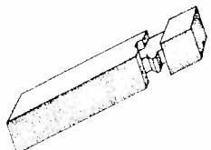
Fig. 6 and 7. A moss hole was criticized by Polhem: "mice will carry away moss and the corner becomes windy." Polhem designed a joint, below, which will become tighter as the logs dry.
