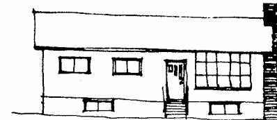
Fig. 3. An un-insulated Canadian bungalow loses about 50% of its heat through the ceiling and 14% through the basement wall. Insulated to 1976 standards it would use about 30% of the fuel and lose 11% of its heat through the ceiling and 31% through the basement wall.
