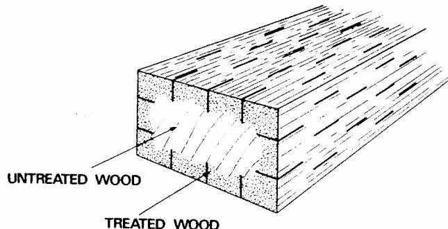
**Fig. 7.** For wood species not easily penetrated, incising enables a uniform shell of treated wood to be created which protects the untreated core.
