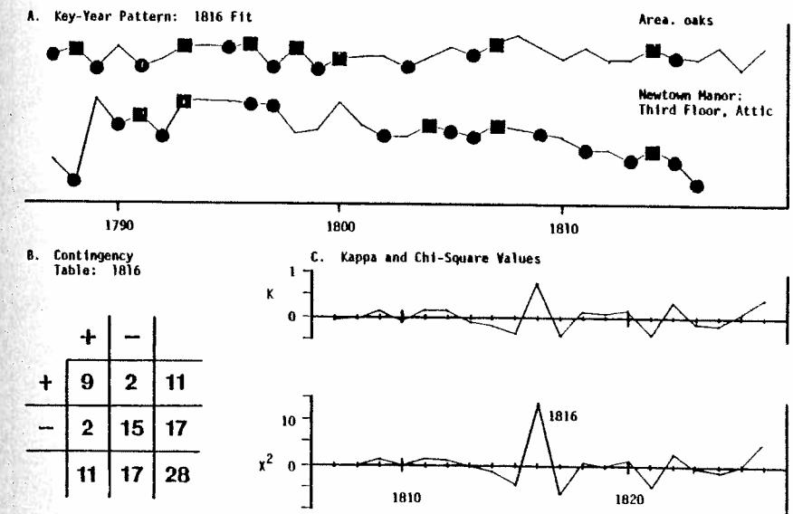
Fig. 5. The cross dating of the key-year pattern ( $P = .05$ ,  $n = 9$ ) for the third floor and attic timbers and rafters of the Newtown Manor House, with the oak key-year pattern. The year of best fit for the last year of tree growth was 1816 ( $X^2 = 13.7$ ,  $K = .7$ ).
