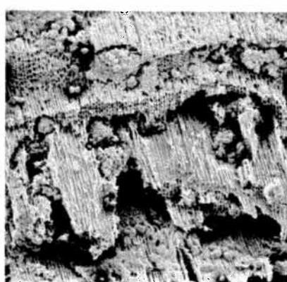
Fig. 22. SEM micrograph of a region of sapwood directly below the weathered surface. The beetles tunnel out selectively thin walled early wood tracheids leaving the stronger late wood tracheids which maintains the integrity of the wood. The tunnels are filled with faecal pellets and frass which are similar to sawdust. Credit M.L. Florian, British Columbia Provincial Museum.
