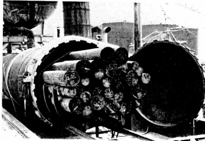
**Fig. 10.** A modern treating retort, with a rapid closing door.
