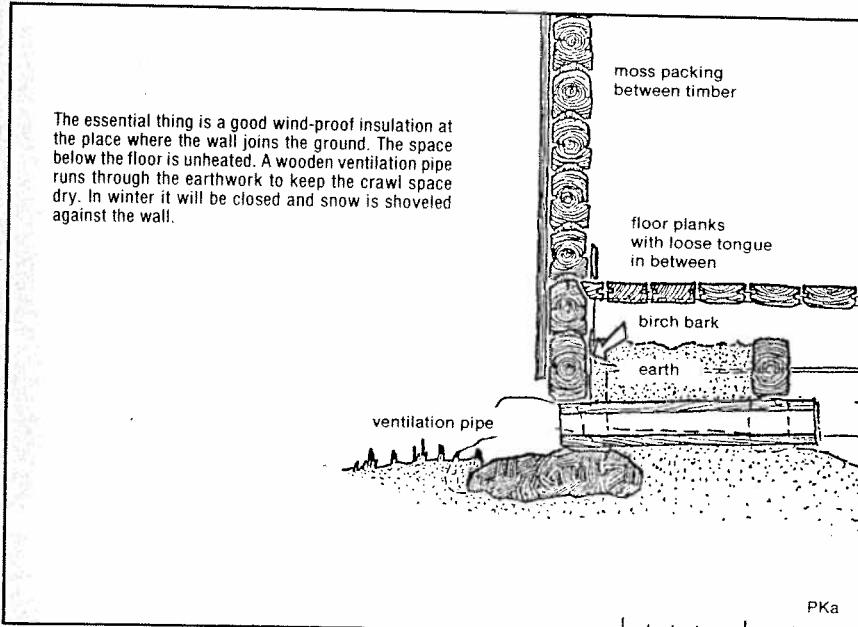
Fig. 1. The floor construction of an 18th century house at Jakkarila manor, Porvoo.
