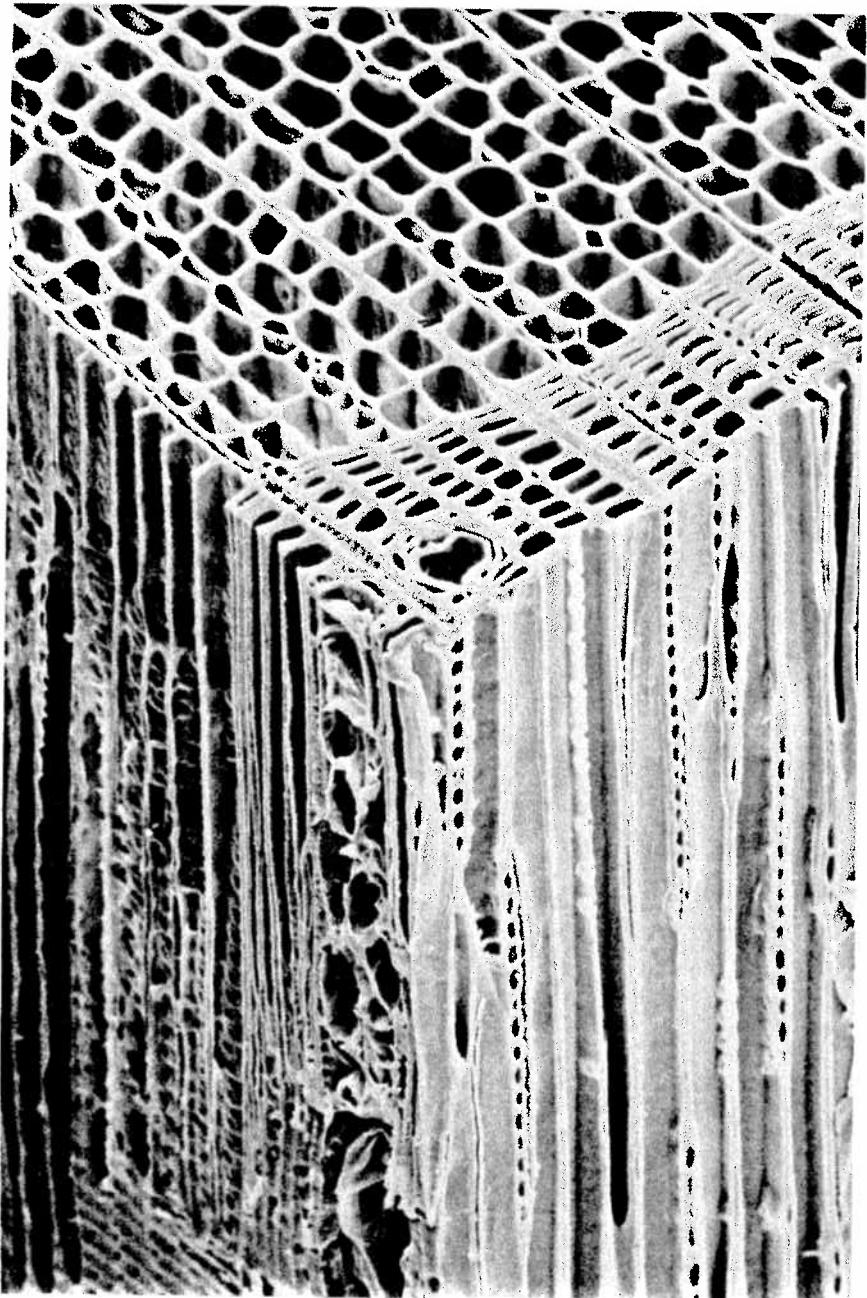
Fig. 4. Wood is not a simple homogeneous medium. It is composed of many tubular cells bonded together and through which preservative solution can flow, passing from one cell to another by way of openings in the cell wall.
