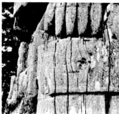
Fig. 23 and 24. These two photographs show the same region on a totem pole but Figure 23 is taken of the southeast side of the pole and Figure 24 the northeast side. The differential weathering pattern is a result of the direction of exposure. The intense weathering is due to wind and rain direction. Credit M.L. Florian, British Columbia Provincial Museum.
