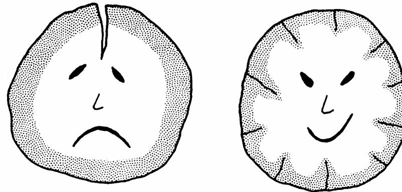
A. Wood too wet before treatment; subsequent checking has passed through treated shell and exposed untreated wood.
