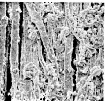
Fig. 21. SEM micrograph of a sample of the tangential weathered surface that is dark grey due to the spores of the fungus *Aureobasidium pullulans*. Credit M.L. Florian, British Columbia Provincial Museum.
