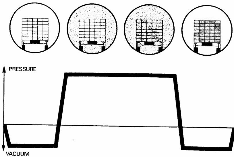
Fig. 13. The full-cell process is used for the pressure treatment of wood with waterborne preservatives.
