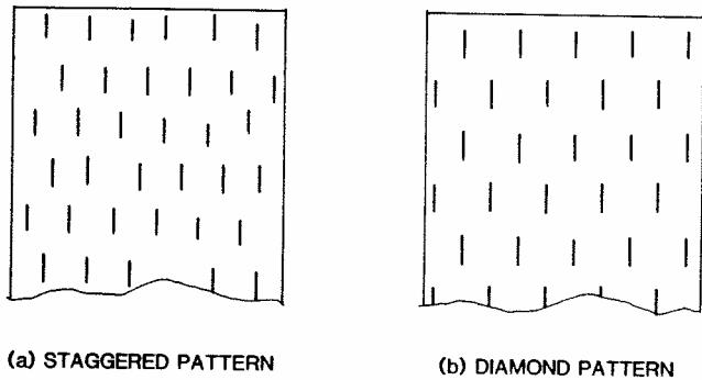
**Fig. 8.** Two basic types of incising patterns are used by the Canadian wood treating industry.
