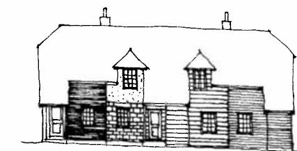
Fig. 2. 'Hydro-stone' houses in Halifax, N.S. with individual owners making cladding decisions in isolation. The original finish is the second from the left, stucco over concrete block.
