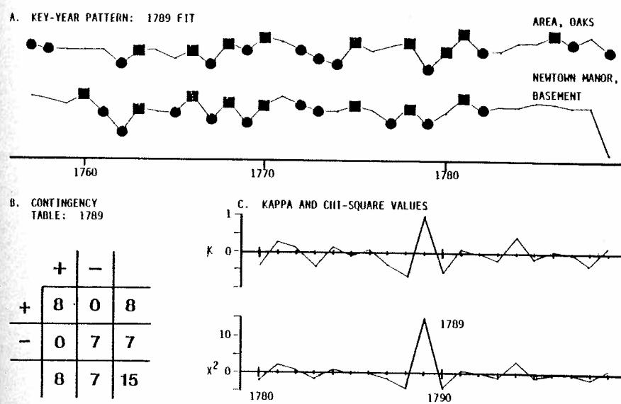
Fig. 4. The cross dating of the oak key-year pattern ( $P = .05$ ,  $n = 16$ ) for the basement ceiling timbers in the Newtown Manor House with the oak key-year pattern. The year of best fit for the year of last tree growth was 1789 ( $X^2 = 15.0$ ,  $K = 1.0$ ).
