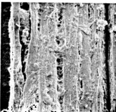
Fig. 19. The surface at the sharp line (running from lower left to upper left) of demarcation in color front grey to white showed no structural difference under SEM. The weathered tangential grain (Fig. 15) shows loss of wood ray cells and consolidation of collapsed wood tracheids. Credit M.L. Florian, British Columbia Provincial Museums\*.
