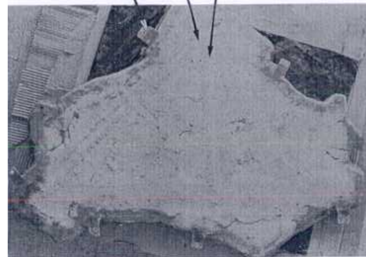
The reverse of the block following its reinforcement with fiberglass mat and polyester resin. Note the mounting brackets and the plastic rods.
