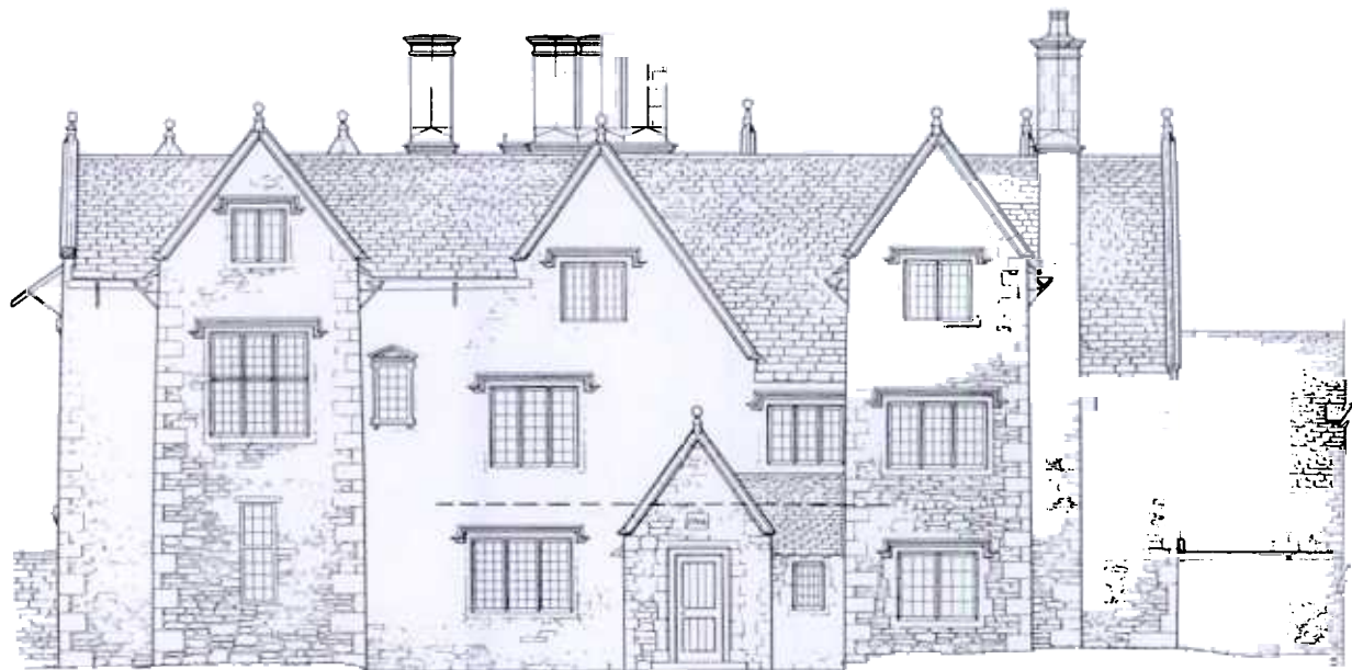
Fig. 15. — The North Elevation as it now is, re-ordered and with the new porch and public entrance. The dotted lines show the position of the reinforced concrete beam inserted length by length to distribute the weight.
