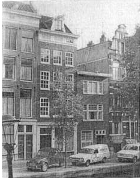
FIGS 11 and 12. 37 Bloemgracht before and after reconstruction in 1977. Unusually, this was a complete rebuilding and replacement of a house that was in poor structural condition and totally out of keeping with its surroundings. It was rebuilt as four residences in a more appropriate style.
