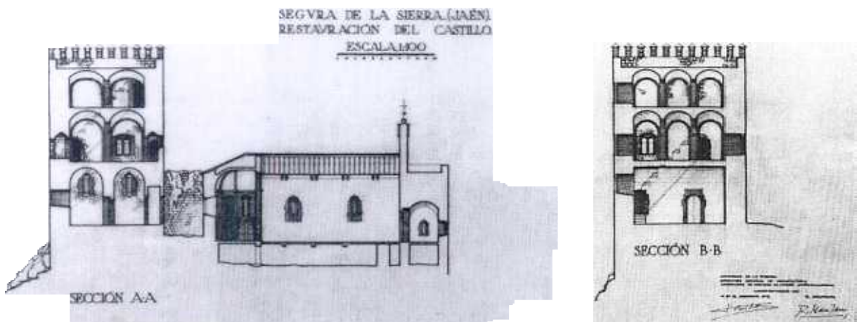
Fig. 12. Sections through "Tower of Homage" and church.
