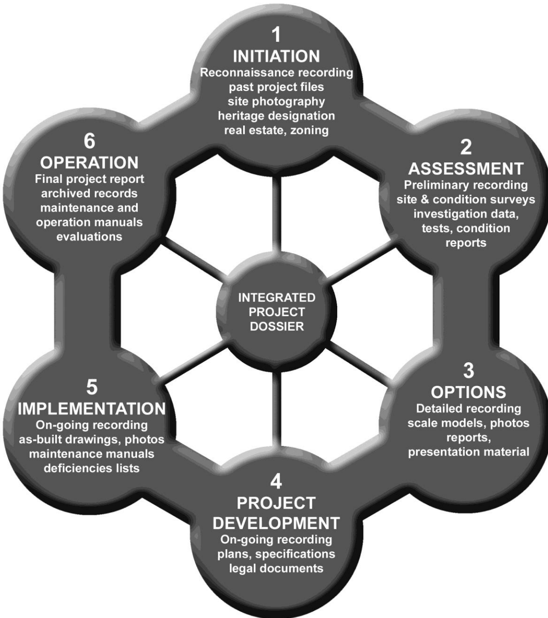
Figure 12 The diagram illustrates the six phases of the Conservation Process with a few examples of typical documentation produced during each phase. Illustration: F. LeBlanc
