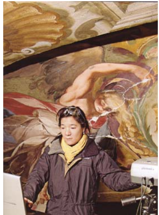
Photo of Lorinda Wong in the J. Paul Getty Trust Annual Report. It shows Lori using multispectral imaging to study the seventeenth-century wall paintings by Andrea Pozzo at the Mission of Mondovi in Italy, as part of the GCI's collaborative Organic Materials in Wall Paintings project
