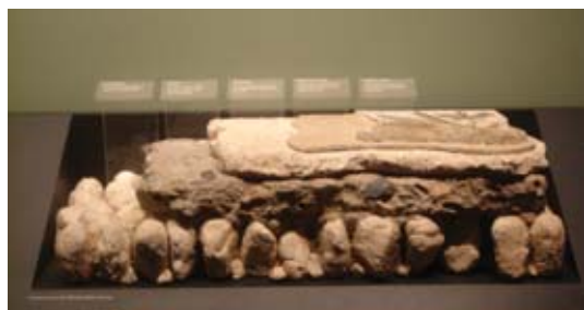
Typical stratigraphy of a Roman mosaic floor displayed in the Getty Villa exhibition entitled Stories in Stone - Conserving mosaics of Roman Africa
